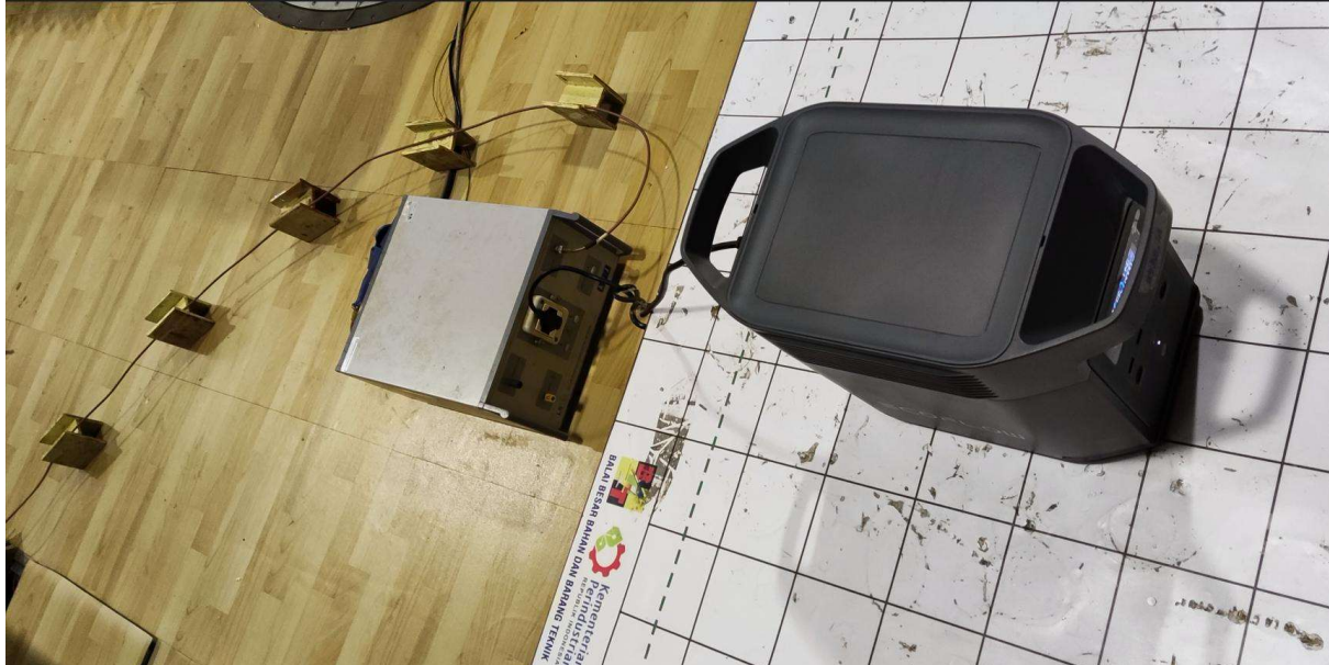
Foto 5. Setting Pengujian Conducted Emissions at Mains Terminal
