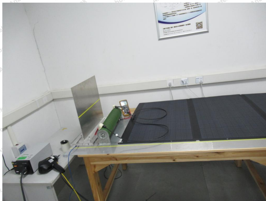
Photo of Electrostatic Discharge Immunity Test
