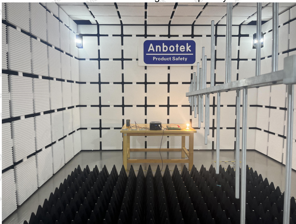
Photo of RF Field Strength Susceptibility Test
