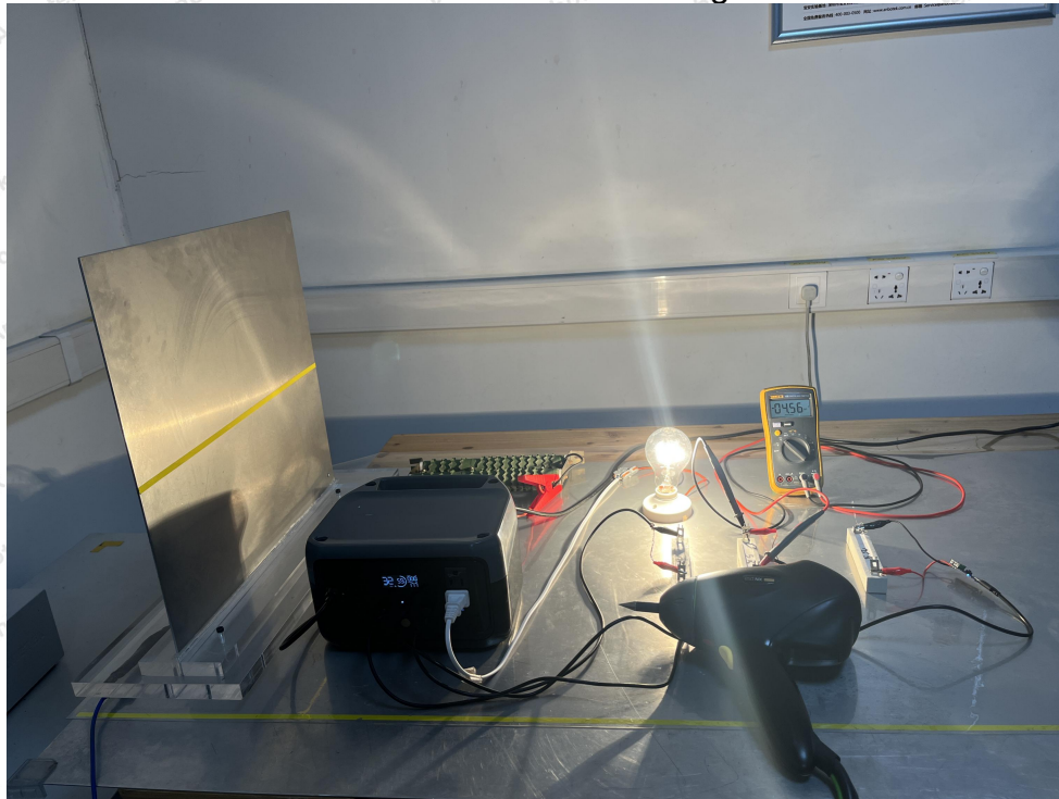
Photo of Electrostatic Discharge Test
