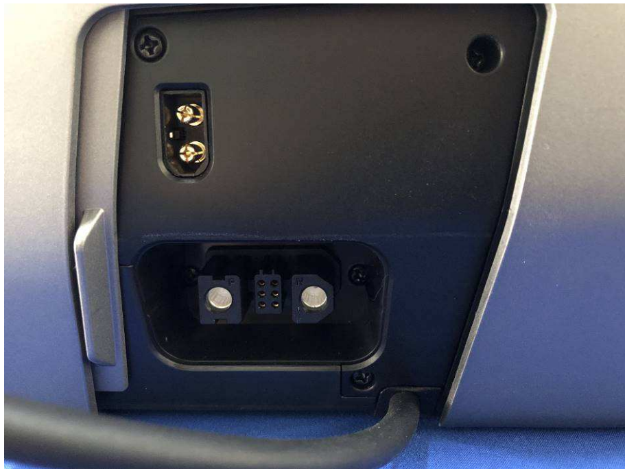
Figure 16. AC Power cord, DC input connector and PV input connector
