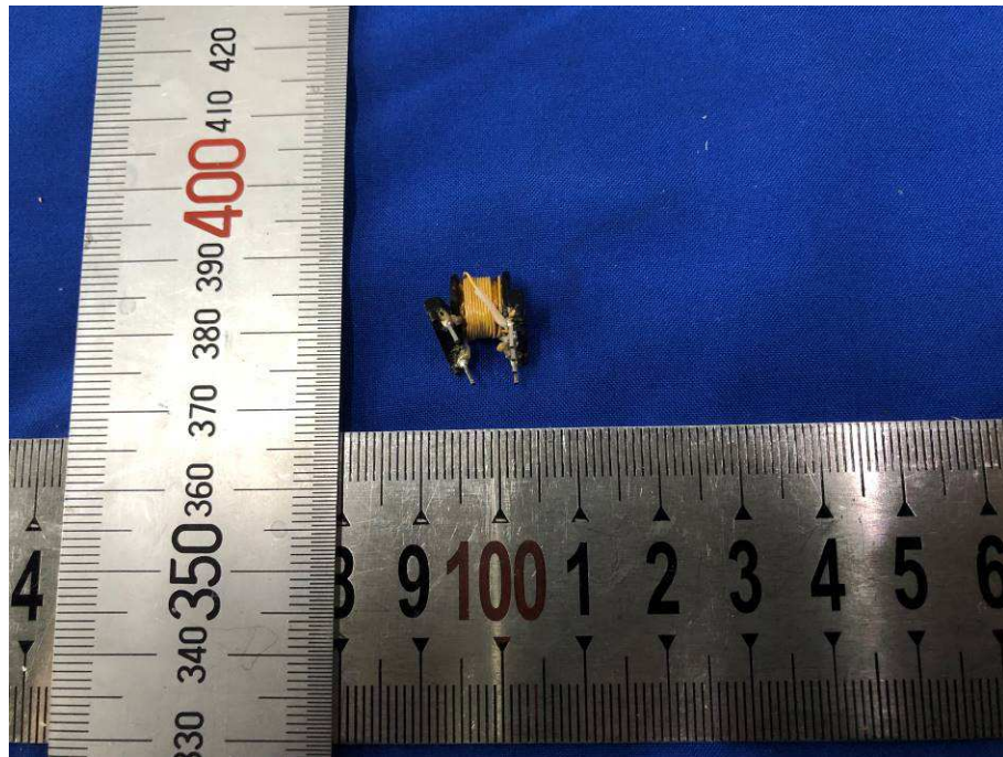
Figure 41. Transformer T1 of main PCB
