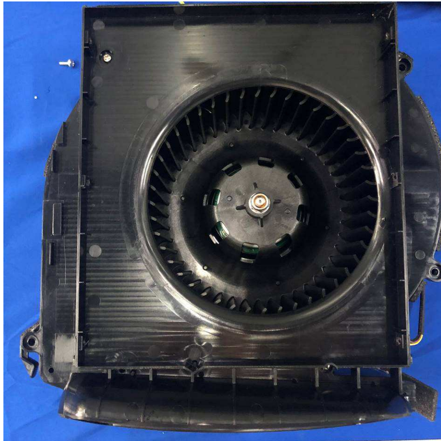
Figure 59. Evaporator fan motor
