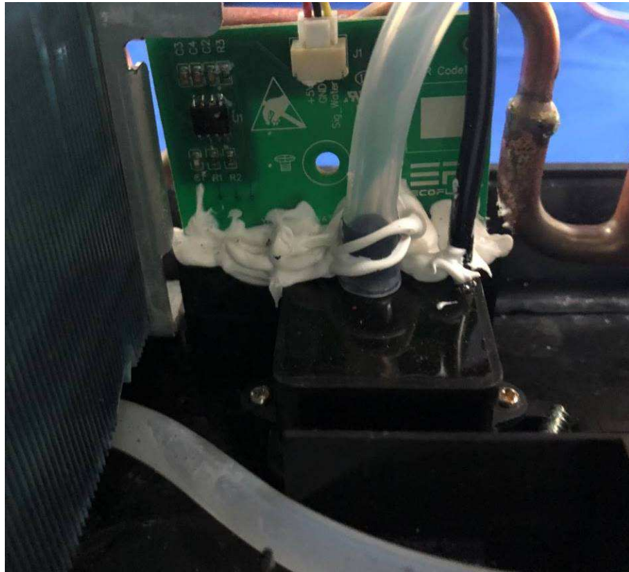
Figure 69. Water pump and water level sensor
