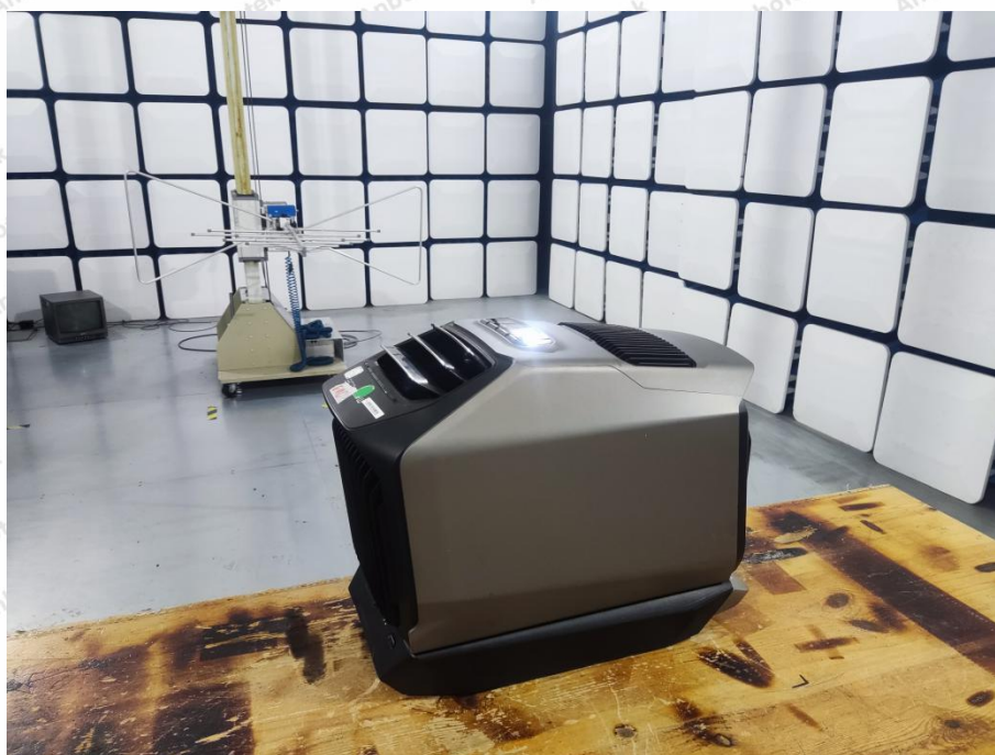
Photo of Radiated Emission Test (Below 1 GHz)
