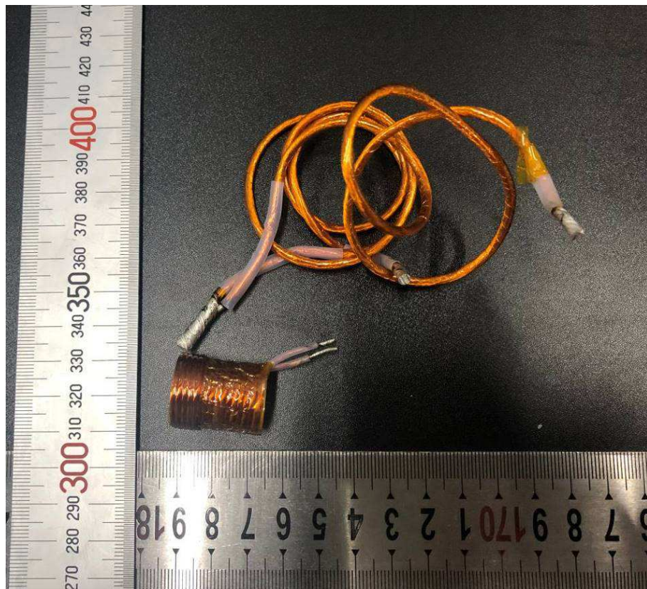
Figure 38. Transformer TX1 of main PCB
