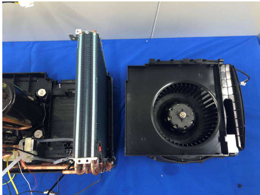
Figure 62. Condenser and condenser fan motor
