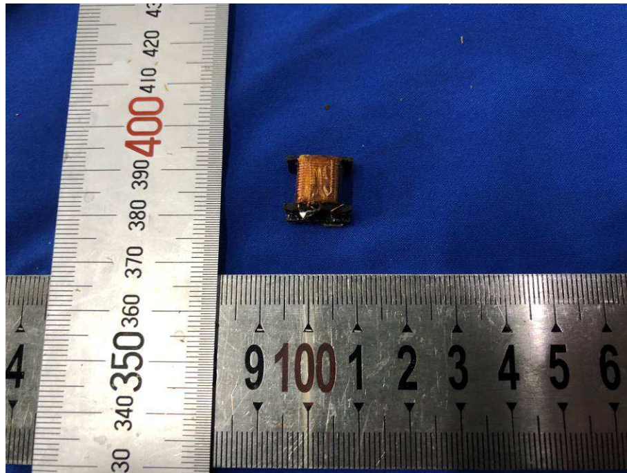
Figure 49. Transformer T2 of main PCB
