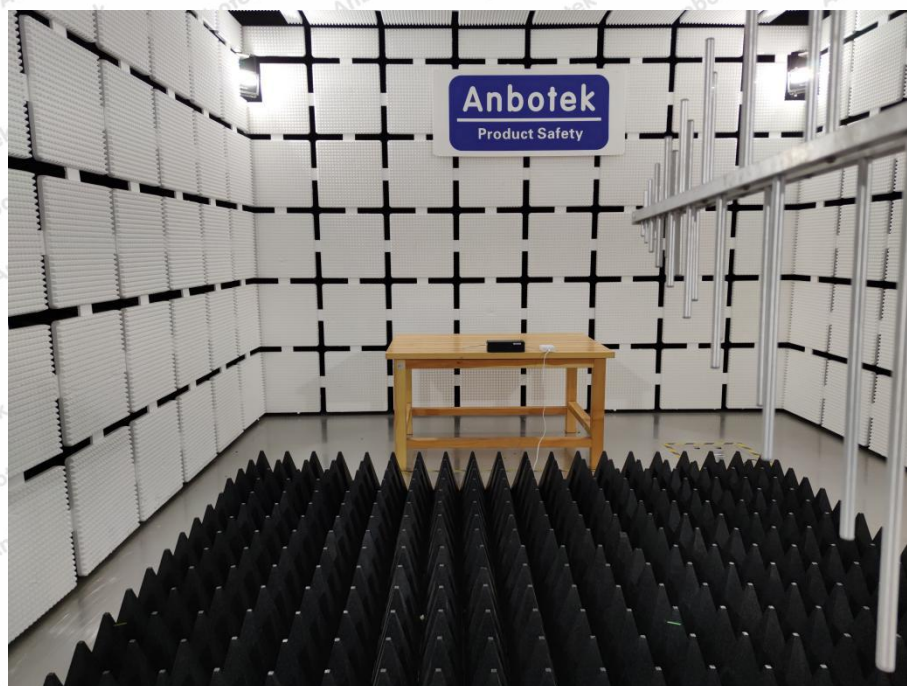
Photo of RF Field Strength Immunity Test
