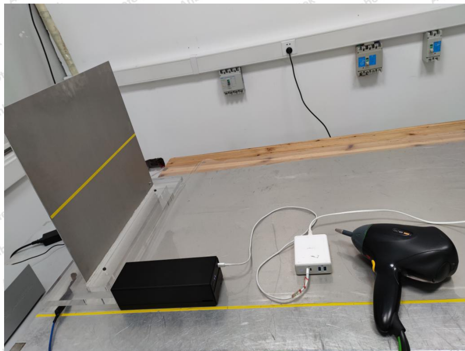
Photo of Electrostatic Discharge Immunity Test
