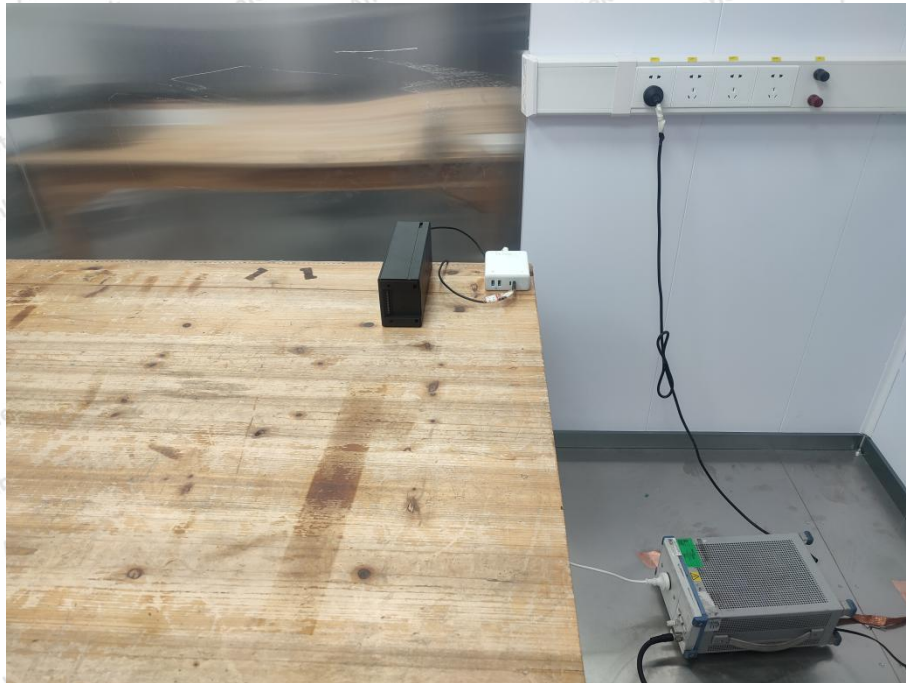
Photo of Power Line Conducted Emission Test
