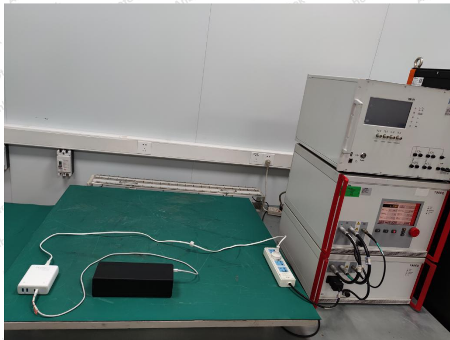
Photo of Electrical Fast Transient/Burst Immunity Test
