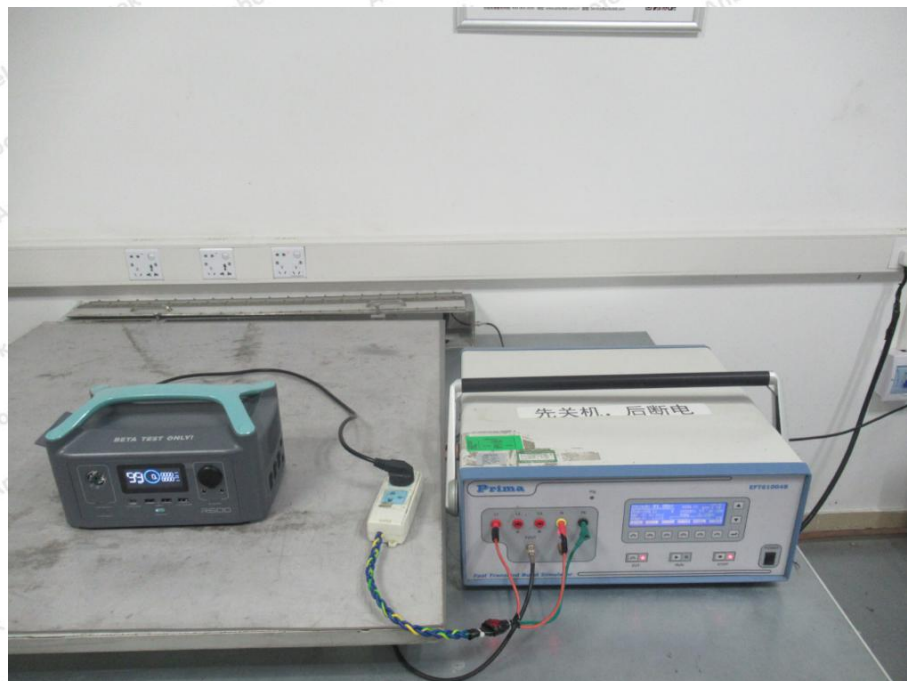
Photo of Electrical Fast Transient/Burst Immunity Test
