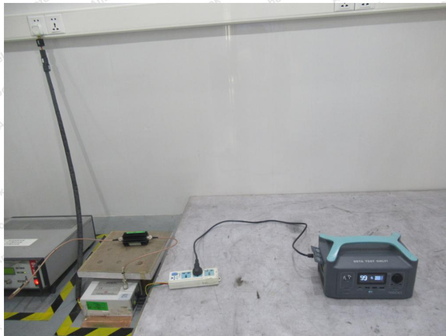
Photo of Injected currents susceptibility Test
