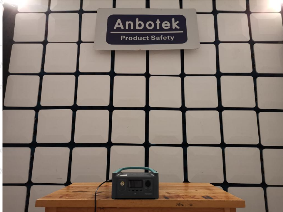
Photo of RF Field Strength susceptibility Test
