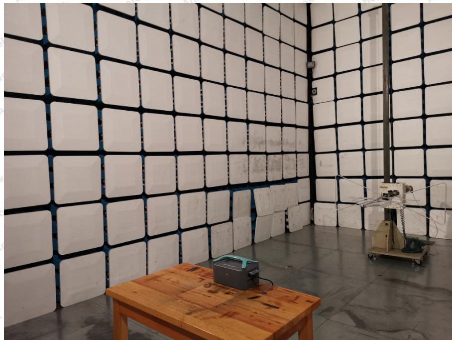
Photo of Radiated Emission Test
