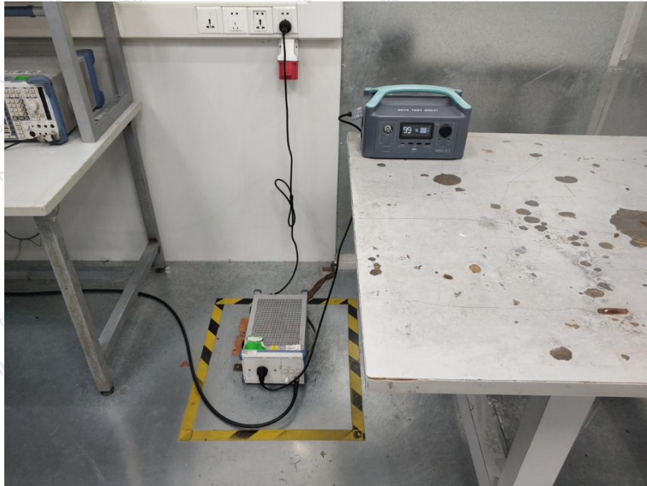
Photo of Power Line Conducted Emission Test
