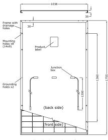
Note: dimensions in mm, tolerance +/- 2 mm
